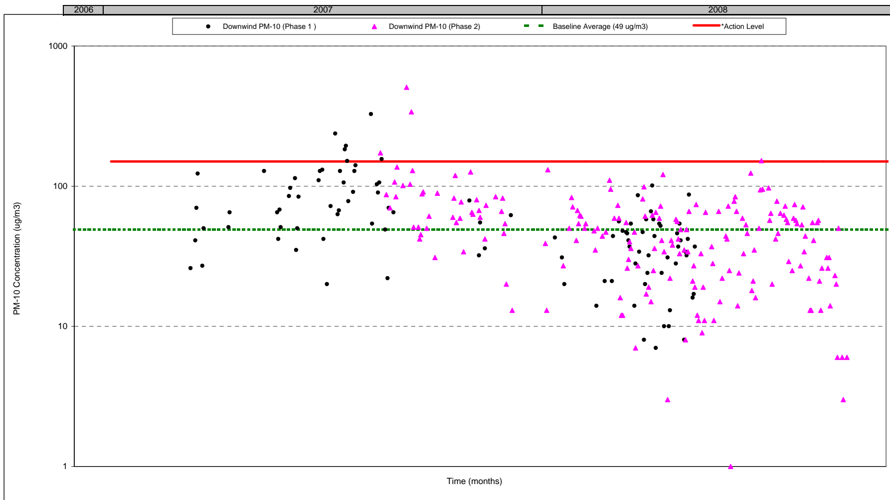
Figure 15 Supplemental Downwind Particulate Matter Concentration Data Community Air Monitoring Completion Report Bay Shore/Brightwaters Former MGP Site February 2009
